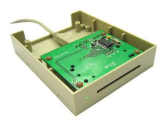
The ACR38F is the ideal solution for easy integration of a smart card reader into the desktop environment. It uses the same electronic circuit as the ACR38, and has the same versatility and cost-effectiveness that have always been associated with ACS smart card readers. Using the USB interface, it uses the PC's internal power supply, and can be configured in several ways to suit the customer's preference.
